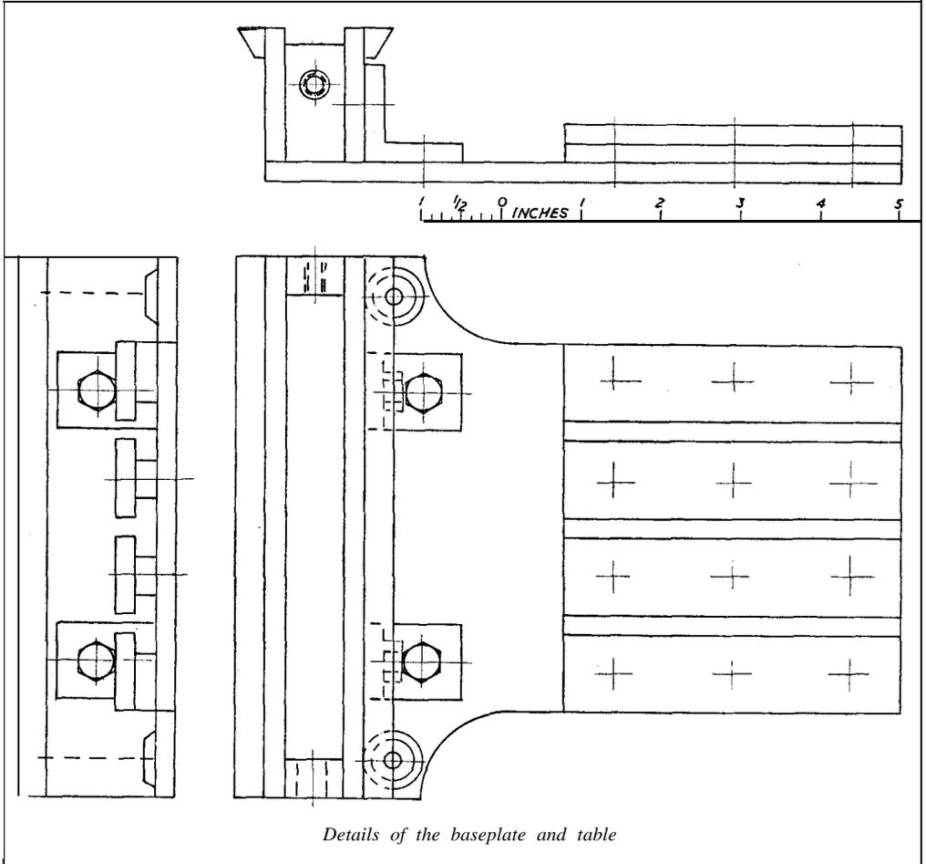
material is used, being shaped to slide fairly tightly between the strips on the front plate. To this back plate another plate is riveted, being drilled and tapped to accommodate the  $\frac{1}{4}$  in. Whitworth feed screw which I turned from a short length of  $\frac{1}{2}$  in. diameter mild-steel bar, starting the thread by means of a tailstock die-holder, and afterwards finishing the thread with hand tackle in the vice.
